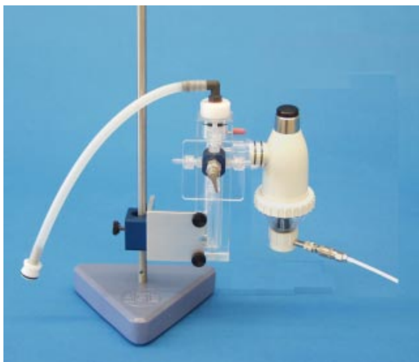
Multigas adapter and connection kit for isolated Mouse lung system IL1, equipped with nebulizer
