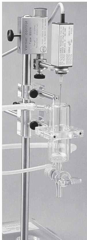
Organ bath (1 channel) Tissue vessel (20 ml) in working position („closed“)
