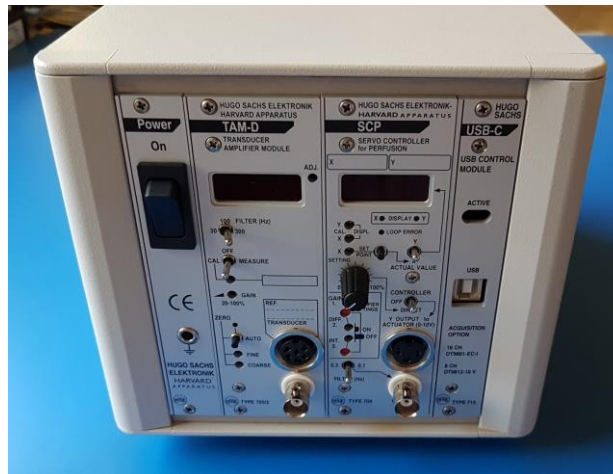
Example 2: TAM-D and SCP installed in a MiniCase housing Type 609 together with an USB-C Control module to record pressure and flow with a Data Acquisition System (DAQ),
