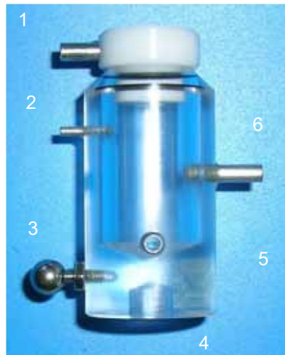
Fig. 4: Bubble trap for the moist chamber.
