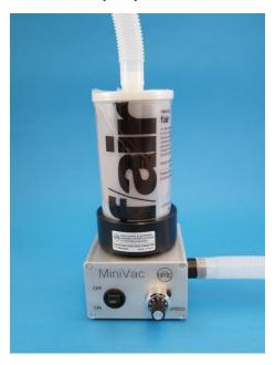
MiniVac shown with a F/Air canister and adapter on the inlet port. In this set up, the isoflurane gas mixture is pulled directly through the F/Air canister, where it is scavenged. F/Air canister, adapter and 22mm tubing is not included.
