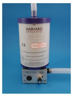
MiniVac shown with a Fluosorber canister and adapter on inlet port.
