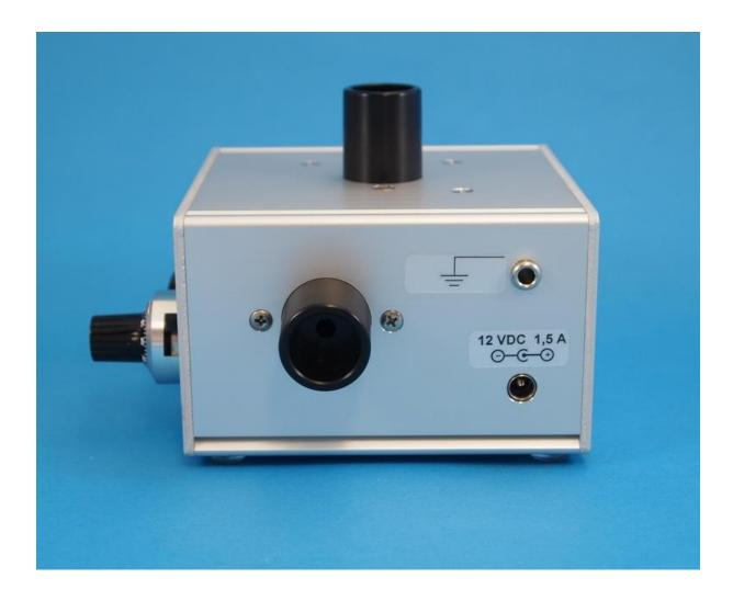
On the right side panel, is the power input for the power supply, the connector for the ground cable as well as the exhaust/out port.
