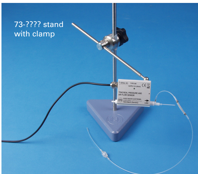
TP/AF sensor mounted on a rod to be connected to an anesthetized, non-ventilated animal.
