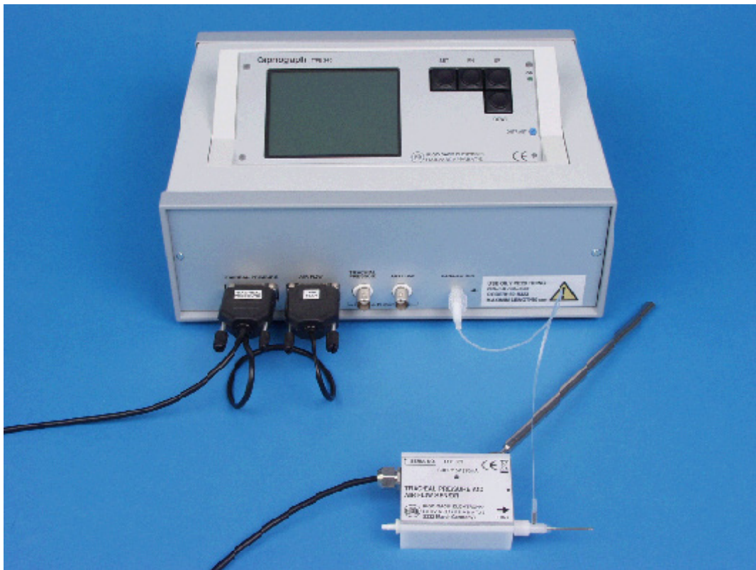
TP/AF sensor connected to the Capnograph without ventilator to be connected to a mouse for a non-ventilated application.
