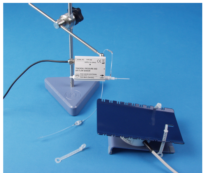
TP/AF sensor mounted on a rod placed next an operating table to be connected to an anesthetized, non-ventilated mouse.
