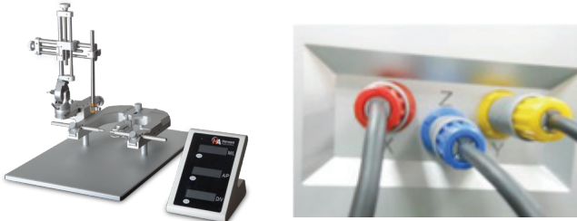
Fig.3 Connection Diagram of each X-, Y- and Z-Axis Sensor to Digital Display Module
