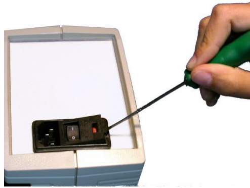
Figure 2. Open fuse-holder door.
