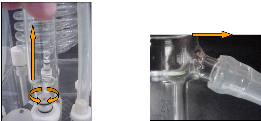
Figure 25. Removing the vessel.
