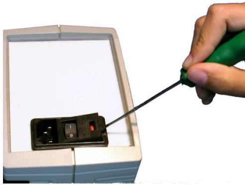
Figure 2. Open fuse-holder door.
