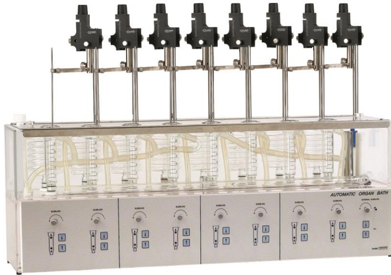
Figure 7. LE01.o86 8-channel Automatic Organ Bath.
