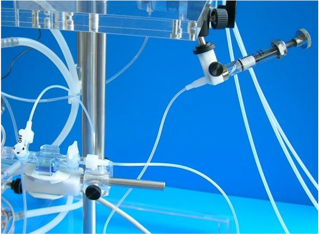
APT300 transducer with spindle syringe and PE catheter, all filled bubble free with degassed water
