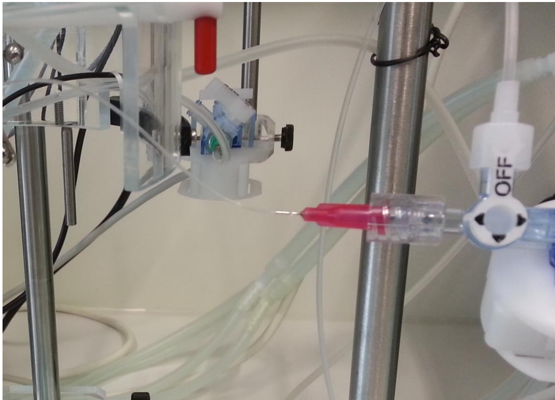
PE catheter attached on red stub needle, Needle attached to APT300 pressure transducer
