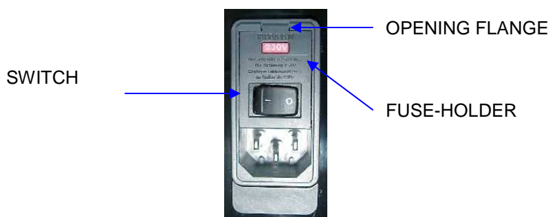
Figure 2. Power inlet, main switch and fuse holder
