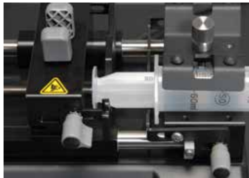
Close-up of syringe positioning with plunger inserted in retaining bracket of pusher block.
