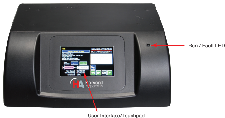
Front view of the PHD ULTRA™ HPSI/XF pump showing important components.
