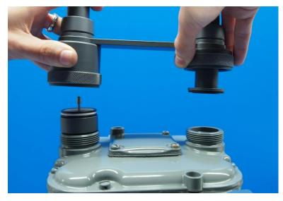
Check the good fit and tighten ferrules by hand
