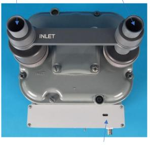
Micro-USB connector for power supply. NO DATA
