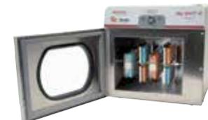
8-Plate Rotator/Incubator with carousel for 96-well Equilibrium Dialyzer plates
