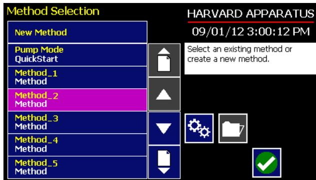
*The EZ PRO™ Method Selection screen showing a button highlighted after a single touch.*
