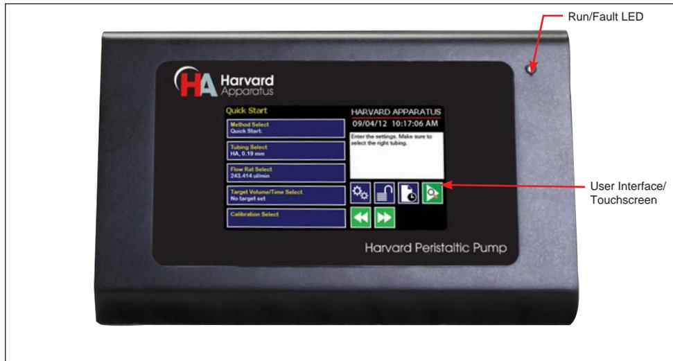
*Front view of the Harvard Peristaltic pump showing important controls.*
